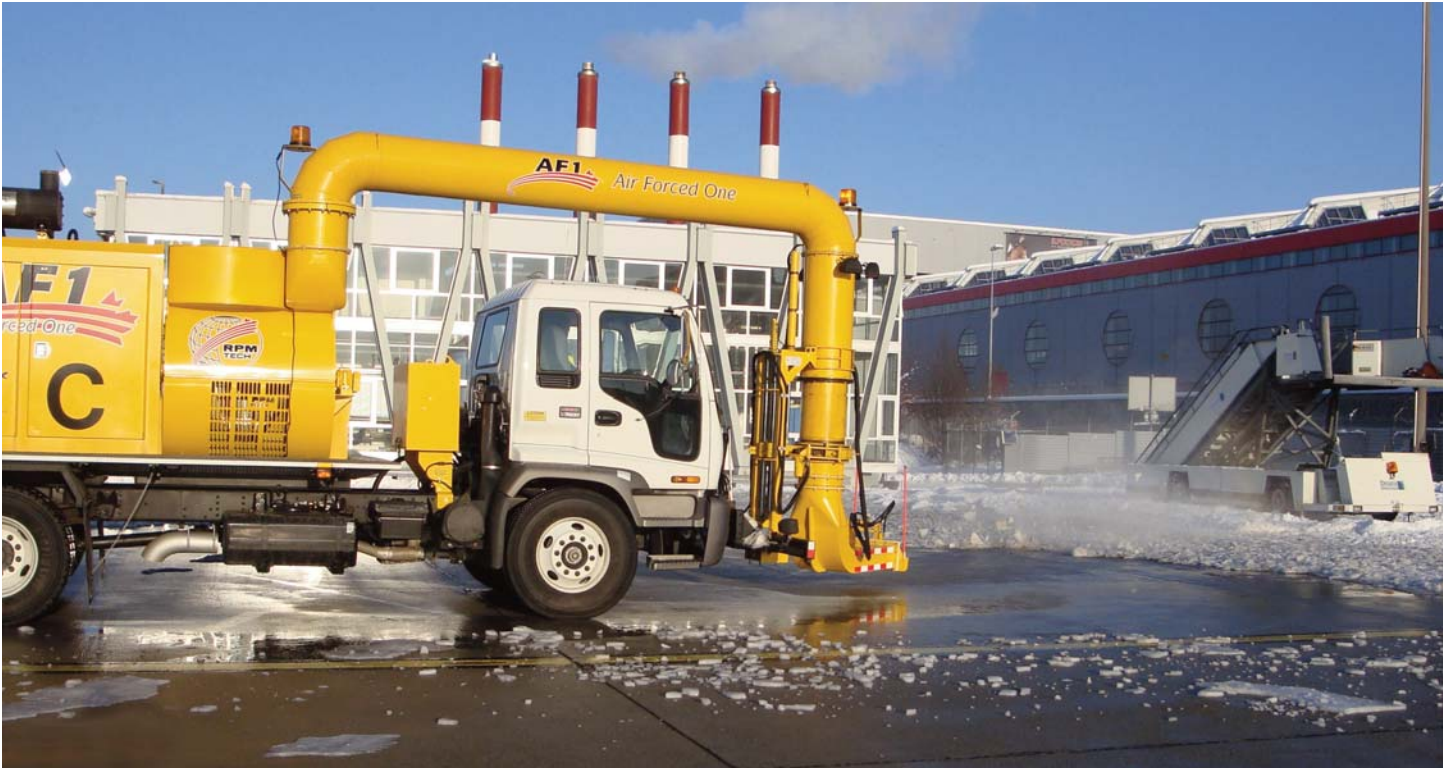
The AF1 cold air blower clearing ice and drying the surface at Geneva Airport, Switzerland.
